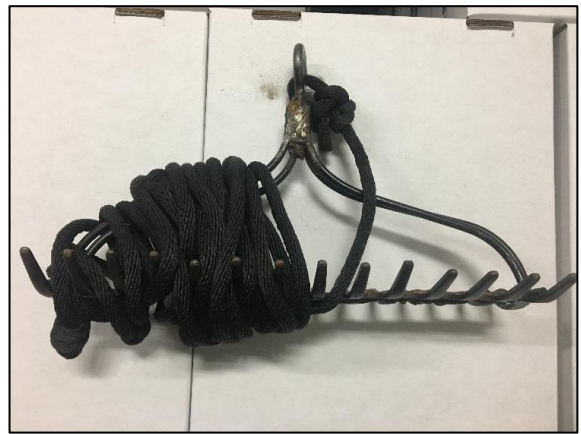
Figure 1 and 3: Double-headed, weighted garden rake, attached to a rope used to survey aquatic vegetation.
