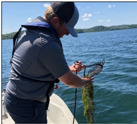
Figure 1 and 3: Double-headed, weighted garden rake, attached to a rope used to survey aquatic vegetation.
